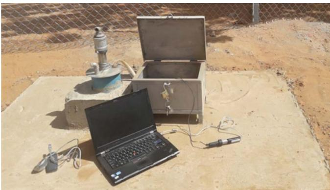
In Darfur, UNAMID successfully established a groundwater monitoring program to monitor the drawdown/recovery parameters of an aquifer, using sophisticated data loggers installed in observation wells within the target aquifers. These data loggers are computer based electronic logs, picking up and recording fluctuations in the groundwater level over time. The program enables UNAMID to monitor the effects of its water consumption on the scarce local resources and adjust, where necessary.
